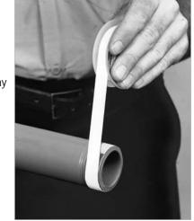
If tape is used, wrap the tape around the entire length of threads beginning with number two thread from the end. The tape should slightly overlap itself going in the same direction as the threads. This will prevent the tape from unraveling when the fitting is tightened on the pipe. Overlapping in the wrong direction and the use of too much tape can affect tolerances between threads. This can generate stress in the wall of female fittings resulting in failure during operations.
