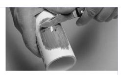
sharp object, drag the edge over the coated surface. Proper penetration has been made if you can scratch or scrape a few thousandths of an inch of the primed surfaces away.
