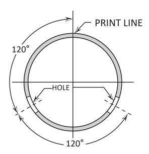
Perforation Specifications: Two rows of 1/2" diameter holes with holes, 5 inches on center.
